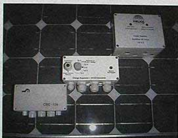
Battery charge controllers tested in the Philippines.
